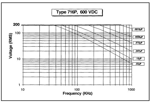
RMS Voltage vs. Frequency @ +85°C
