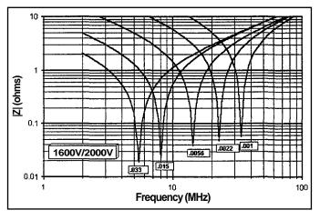
Please note: Capacitance values above are in  $\mu$ F. The resonant frequency and impedance shown above apply to units with a 0.250" lead length and are typical values only. Please contact us for data on the 100VDC rated units.
