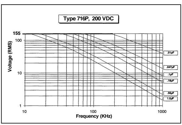
RMS Voltage vs. Frequency @ +85°C
